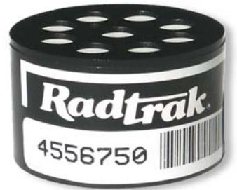
Radtrak measures the average radon concentration at the location of the detector during the monitoring period. The alpha-track detector has, inside the plastic housing, a radiosensitive element that records alpha particle emissions (alpha tracks) from the natural radioactive decay of radon.
