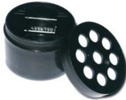
When the detector is returned to Landauer's laboratory, the alpha tracks are counted using computer-assisted image analysis equipment. The number of alpha tracks along with the deployment time period provides the basis for calculating the average radon concentration. The report with the radon gas measurement, reported in picocuries per liter of air (pCi/l), is mailed within seven to ten days after receipt of detector.
