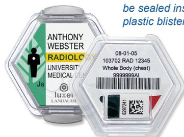
*The Neutrak dosimeter can be sealed inside the Luxel+ plastic blister pack.*
