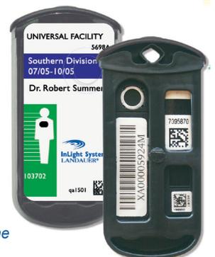
*The Neutrak dosimeter can be enclosed inside the InLight holder.*
